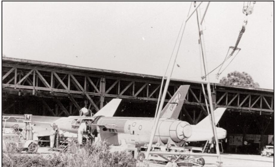
In the late 1950s and early 1960s, the United States Air Force used the Regulus II target missiles as target drones for anti-aircraft training at Eglin Air Force Base. The drones were launched from the Venice airport, not far from where Maxine Barritt Park is today, for the target practice. The 50-foot long missiles with 21-foot wingspans were manufactured by Chance-Vought Aircraft Inc. in Dallas, Texas.
